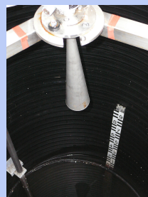
Figure 2. The radar sensor, CS476, operating at 26 GHz.
