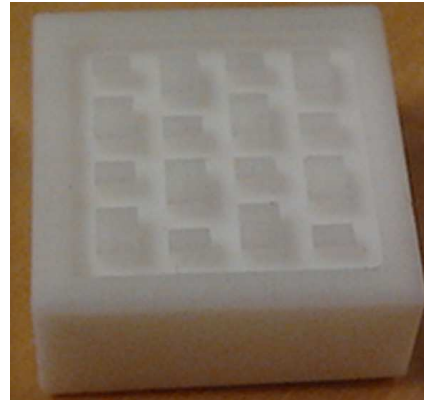
3.7.1 (b) PTFE mold with an area-ratio of 1:2.6.
