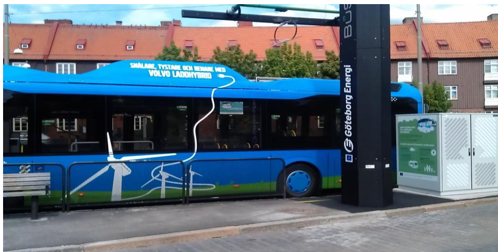
Figure 1. A project bus stop station equipped with the charging facilities [3].
