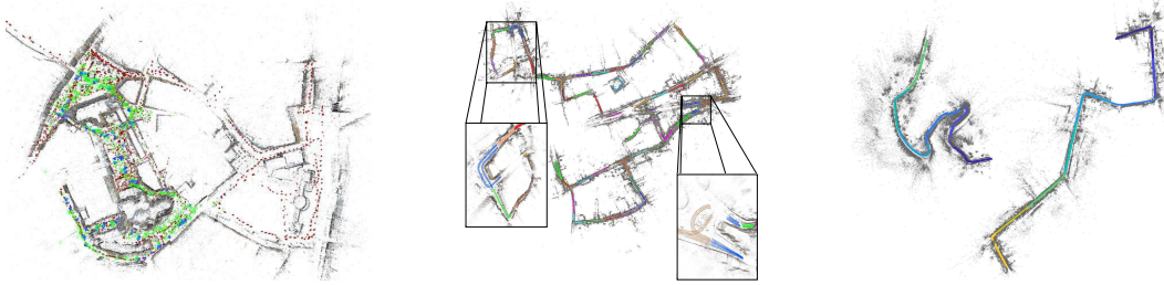
Figure 3. 3D models of the Aachen Day-Night (left, showing database (red), day-time query (green), and night-time query images (blue)), RobotCar Seasons (middle), and CMU Seasons (right) datasets. For RobotCar and CMU, the colors encode the individual submaps.
