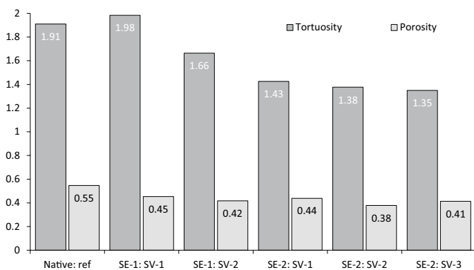
Fig. 7 Porosity and tortuosity for all samples. Porosity was obtained from the available fluid volume fraction, and the tortuosity was obtained by random sampling of streamlines in the flux field
