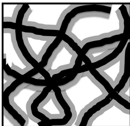
Fig. 3 A schematic visualization of the larger obstructive effect on mass transport from the solid phase, which can result if the cellulose fibrils are swollen (grey) by absorbed [C2mim][OAc], compared to the effect from compact fibrils (black), without [C2mim][OAc]
