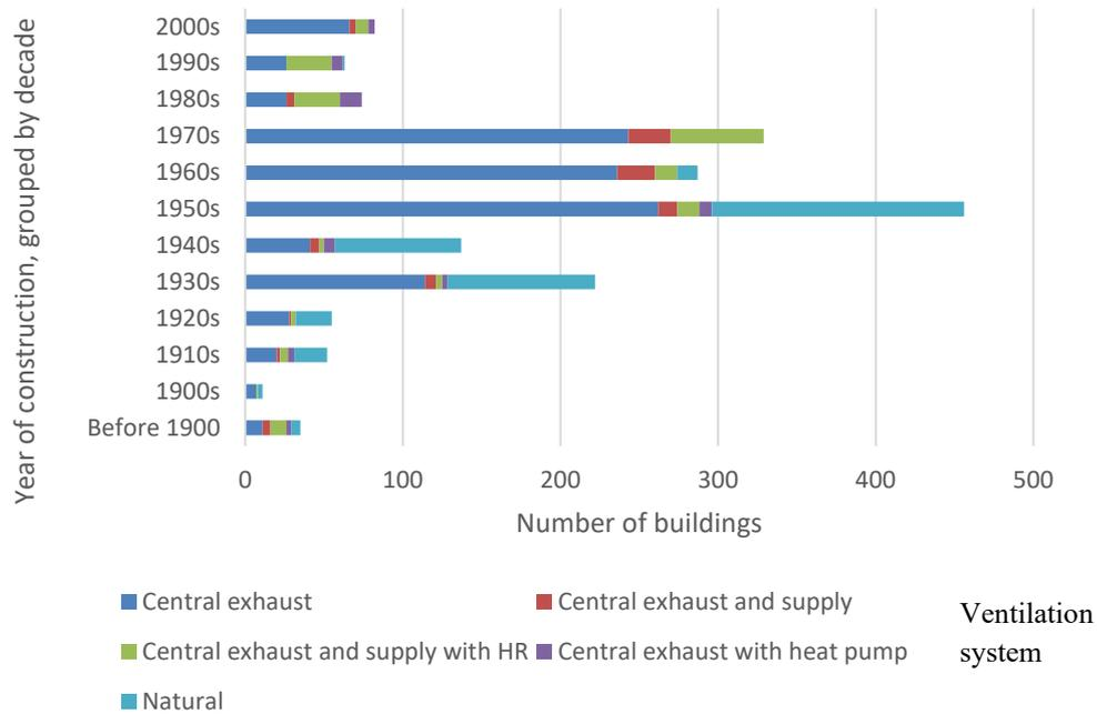
**Figure 9 - Distribution of ventilation systems for buildings in the municipal housing stock grouped by year of construction.**
