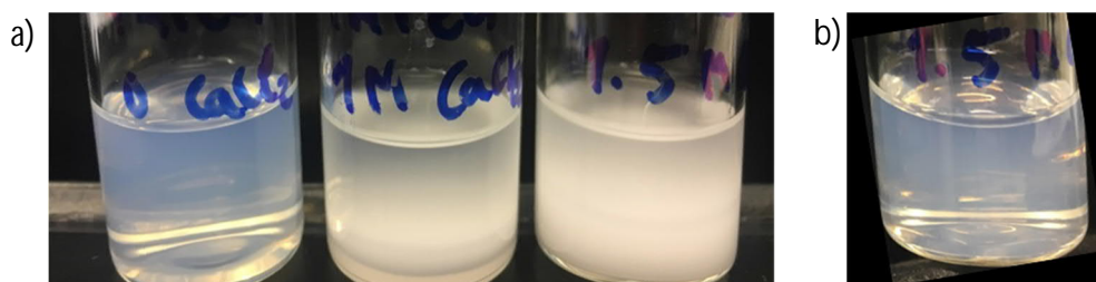
Figure 28. a) Diluted suspensions of \text{mPEG}_{0.74} -SiNP with no added salt, with 1 M \text{CaCl}_2 and with 1.5 M \text{CaCl}_2 , from left to right, at 3.5 wt% of \text{SiO}_2 . The samples have been heated to 110 °C and clouding was observed for the two samples containing \text{CaCl}_2 . b) Shows the sample with 1.5 M \text{CaCl}_2 cooled to room temperature, and the original turbidity was regained.
