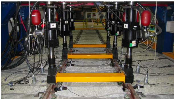
Figure 6.2: Assembly of geotechnical test rig at CEDEX. From [66]
