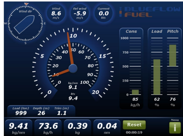
Fig. 2 Interface of the onboard monitoring energy system
