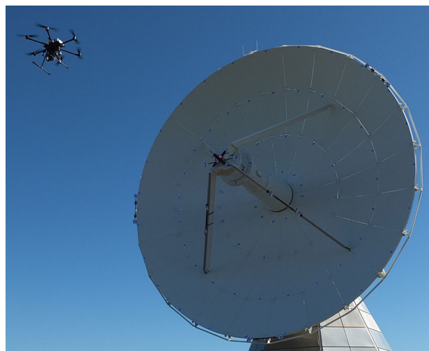
Fig. 3 ONSA13NE during the UAV measurement campaign. The telescope is equipped with photogrammetric targets, coordination cross at the sub-reflector, and scale-bars located at the sub-reflector, the strut elements, and at the rim of the main reflector. The UAV (HP-TS960) carrying the photogrammetric camera is visible in the upper left corner of the photo
