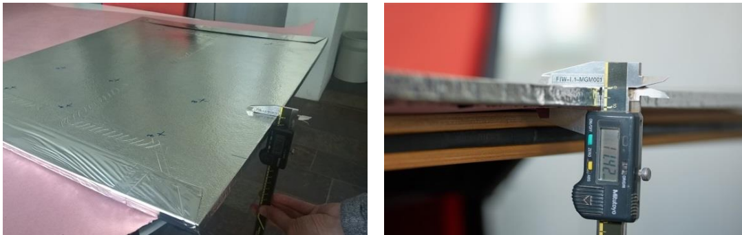
Figure 120: Setup for thickness determination on VIP with ME 2. Source: FIW München.
