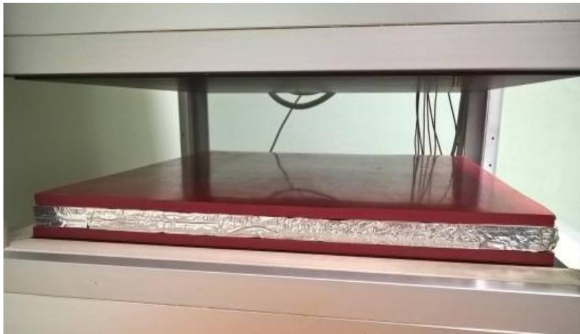
Figure 15: Extra layers of 10 mm thick para rubber. Source: iNRiM.
