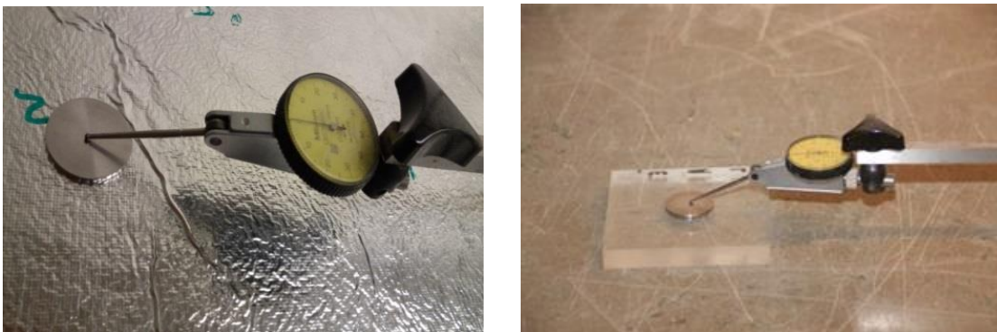
Figure 20: Measurement gauge for determination of panel thickness using a measuring plate (left) or additional rectangular plates (right). Source: KTH Royal Institute of Technology.
