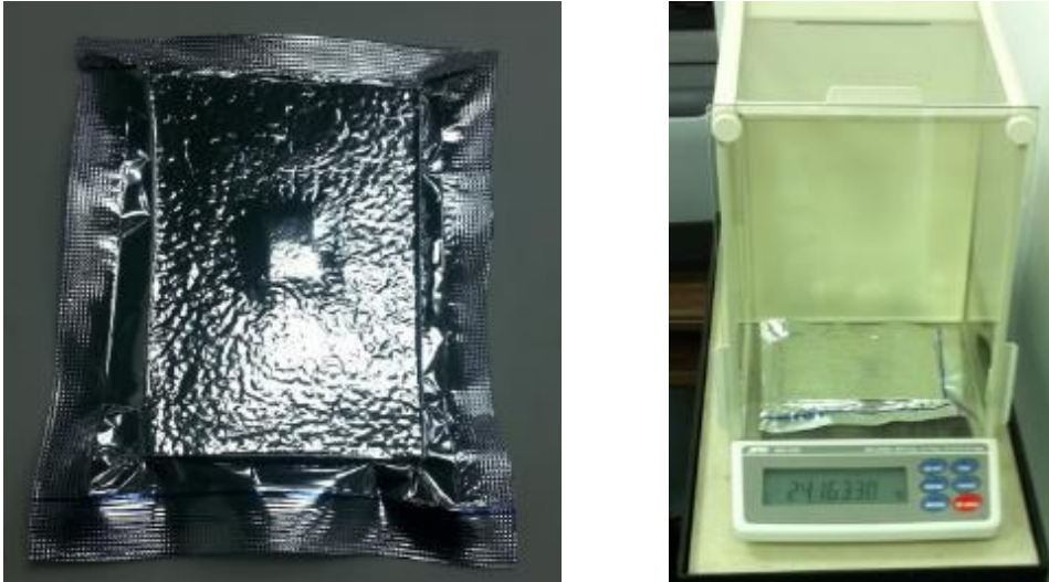
Figure 66: Small panel (~15 cm x 12 cm) with glass fibre and desiccant (left); weighing the panel with an analytic balance (right) (Shufer, 2017).
