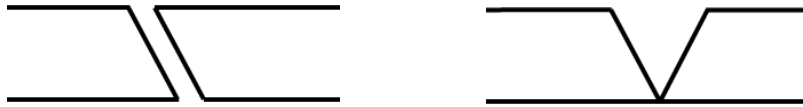
Figure 53: Setup of panels with non-rectangular edge resulting in a small gap (left), and panels with non-rectangular edge resulting in a wide gap (right). Source: FIW München.
