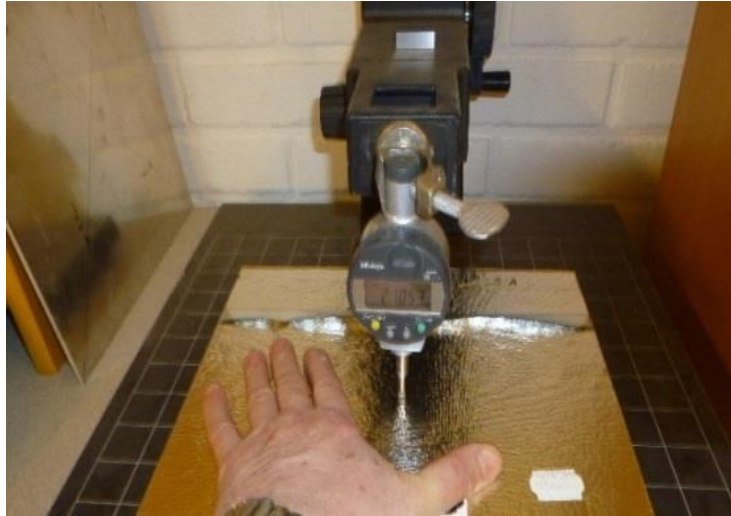
Figure 19: Measurement of thickness using a micrometer measuring gauge. The sample is pressed flat by hand that may cause differing pressure on the surface of the panel. Source: Chalmers University of Technology.
