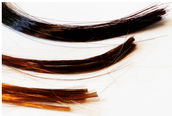
Figure 9.7: Photograph of three cellulose-lignin fibers. Top: 67, Mid: 33, Bot: 10 wt% lignin.
