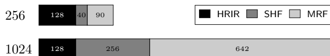
Figure 2: Automatically assigned FIR-filter taps for exemplary rendering configurations at two different block lengths.
