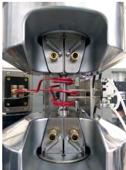
Figure 3. Experimental setup for high temperature biaxial testing
