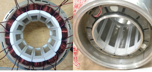
Fig. 4: Wound stator non-drive-end before (left) and drive-end after (right) potting. The oil cooling channels can clearly be seen as formed by the empty space between coils.
