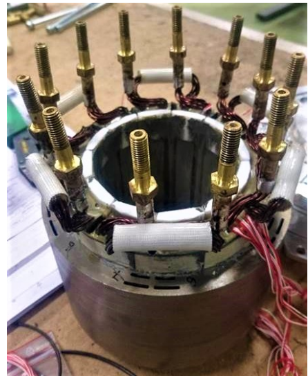
Fig. 12: Stator of 48 V machine after potting and after connection of adjacent coils
