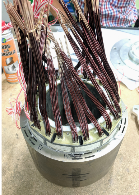
Figure 3.11: 48 V machine during manufacturing, stator without housing and before assembly of phase connection terminals. Each coil has 3 turns of 9 parallel strands 1.5 mm enameled copper wire.
