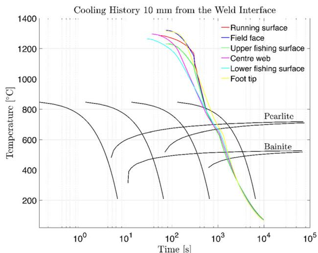
**Fig. 16** Cooling curves for different points in rail cross section and CCT diagram for R260 steel (constructed by JMatPro)
