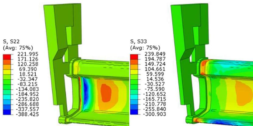
**Fig. 10** Calculated development of stresses with time at weld center after pouring, forging starting 2 min (120 s) after pouring and ending at 2 min 30 s (150 s). Conventional ATW, left, and for the ATW process with additional forging (ALFONS module), right
