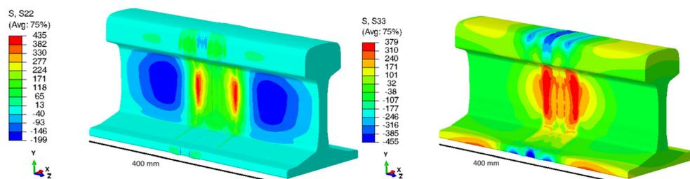
**Fig. 14** Calculated variation of residual stress in the rail mid plane at the weld center (left) and at a distance 50 mm from the weld center line (right). *S*11 is transverse, *S*22 is vertical, and *S*33 is longitudinal stress
