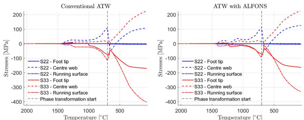
**Fig. 12** Calculated residual stress (MPa) field after conventional ATW process. S22 is vertical and S33 is longitudinal stress component
