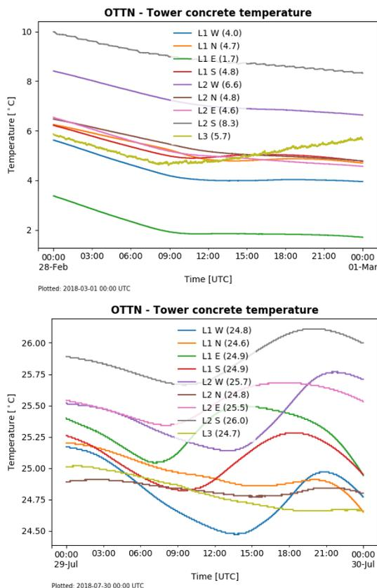
**Fig. 3** Temperatures recorded in the OTT-N concrete tower on 1 March (upper plot) and 30 July (lower plot), which were the coldest and warmest days in 2018. There are temperature sensors on three levels, L1, L2, and L3, where the first two levels have sensors in four different azimuth directions. Similar plots are available for OTT-S.
