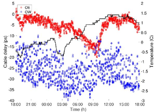
**Fig. 2** Cable measurements performed with the two CDMS systems during VGOS session VT847. While the data for OE (red) show a clear relation to outside air temperature (black line, right scale) and have an RMS of 7 ps only, the data for OW (blue) are much more noisy with an RMS of 27 ps.
