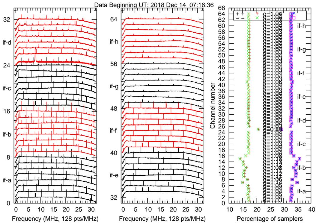
**Fig. 1** Spectra of all 64 channels recorded during a VGOS scan. Black and red lines indicate H- and V-polarization, respectively. Phase-cal tones every 5 MHz are visible in all channels, but the amplitudes decrease for the higher frequencies. The sampler statistics are shown in the right graph. Disturbance due to RFI is clearly visible in the first 16 channels (if-a and if-b), which cover 3.0–3.5 GHz.
