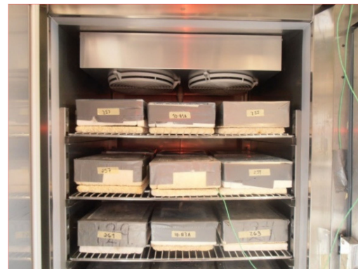
Figure 7. Preparation of salt-frost scaling tests. Left: Application of the rubber cloth and silicone sealant on the test specimens; Right: Salt-frost scaling test specimens placed in the climate chamber.
