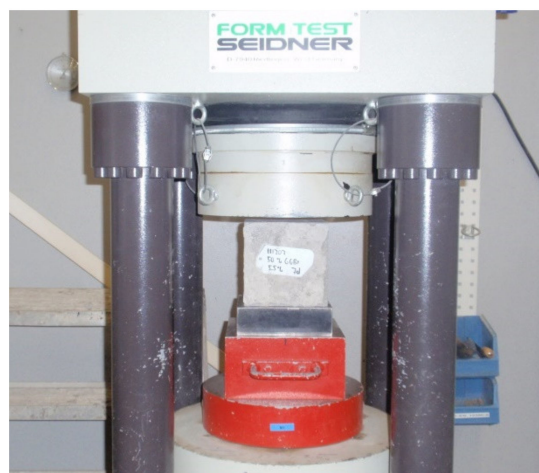
Figure 9. Compressive strength test set-up.
