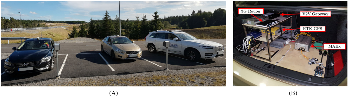
FIGURE 3 Photos of the experimental hardware platform. A, Shows the three vehicles used, B, shows the hardware installation in one of the vehicles. The 3G router was used to provide an IP link for the real-time kinematic corrections used by the GPS receiver [Colour figure can be viewed at wileyonlinelibrary.com ]
