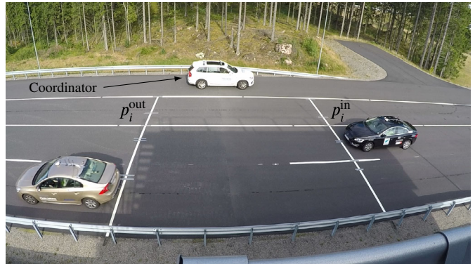
(B) Photo of the parallel configuration used in the experimental validation. The white lines mark the beginning and end of the intersection, p_i^{\text{in}} and p_i^{\text{out}} , and collisions are thereby avoided when only one vehicle is between the two white lines at a given time.
