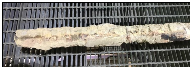
Figure 67: Air-cooled probe exposed 1000 h in the Sulfur Recirculation line (first) and 1000 h in the reference line (after).
