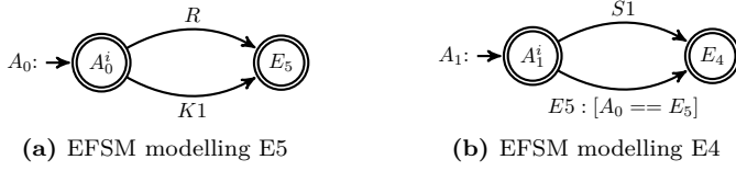
Figure 3: EFSMs for intermediate failure events, E4 and E5 of the fault tree
