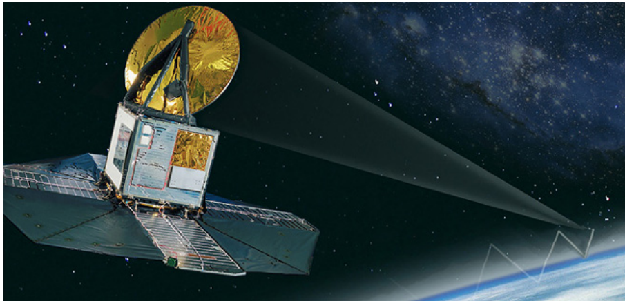
Figure 3.2: Upward and downward scanning of the atmosphere by Odin/SMR.
