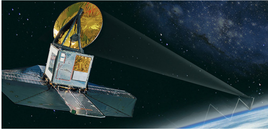
Figure 3.2: Upward and downward scanning of the atmosphere by Odin/SMR.
