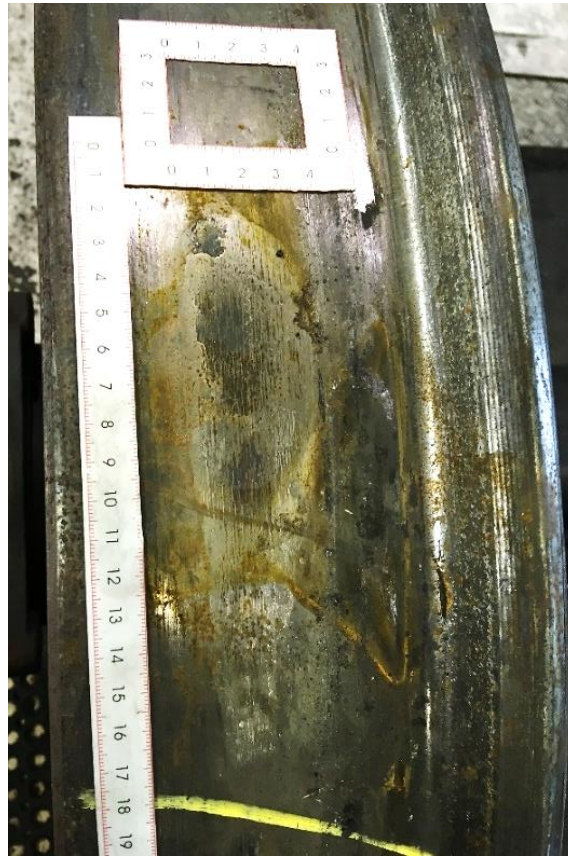
Figure 6: Wheel with a long wheel flat
