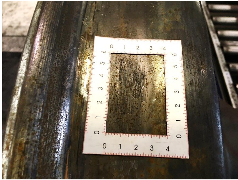
Figure 7: Wheel with a small wheel flat
