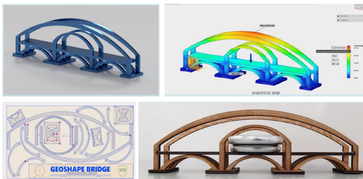
Figure 2. Example of a wooden bridge project (example of student work courtesy of Mr. Edward-Joseph Cefai)
