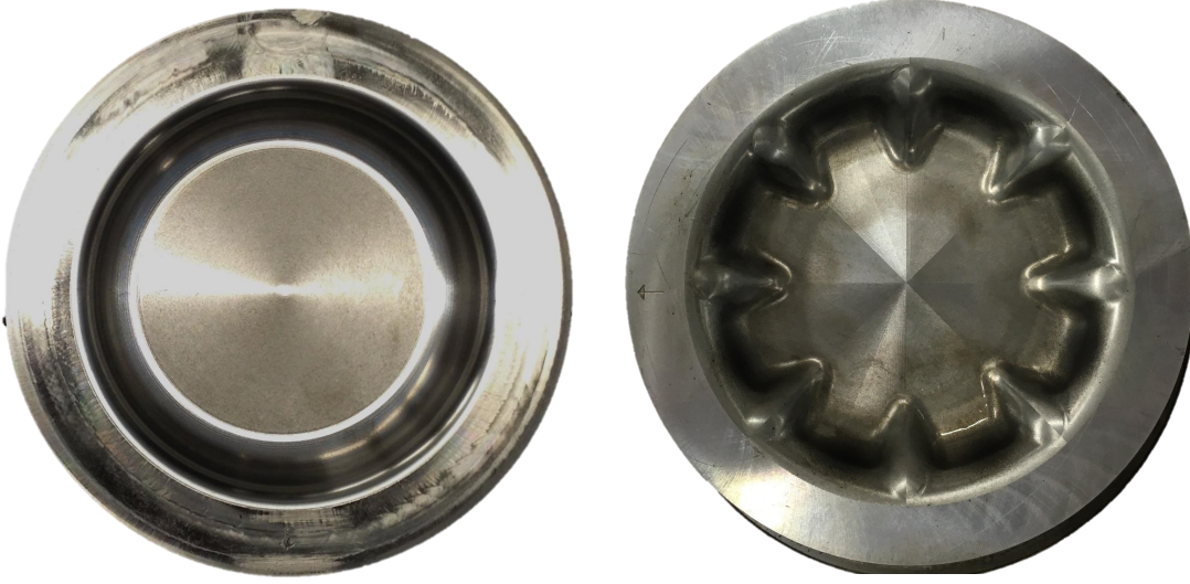
(a) FFlex standard-piston used during the experiments.
