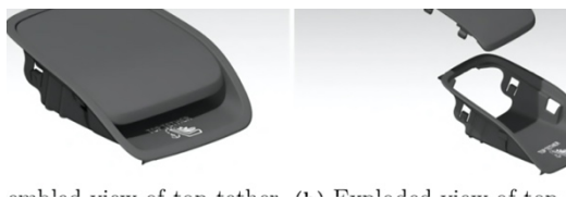
Fig. 2. Components-level views of the top tether.
