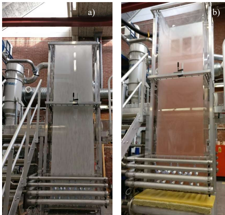
Figure 6. Photographs of the: a) cold-flow scale model with non-scaled particles (glass particles); and b) cold-flow scale model with scaled particles (copper).
