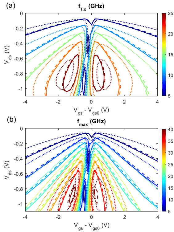
Fig. S8 Influence of the interface trap density on RF figures of merit: (a)  $f_{T,x}$  and (b)  $f_{max}$ . Solid lines correspond to a  $N_{it} = 0 \text{ eV}^{-1} \text{ cm}^{-2}$ ; dashed lines to  $N_{it} = 10^{12} \text{ eV}^{-1} \text{ cm}^{-2}$ ; and dotted lines to  $N_{it} = 10^{13} \text{ eV}^{-1} \text{ cm}^{-2}$ .
