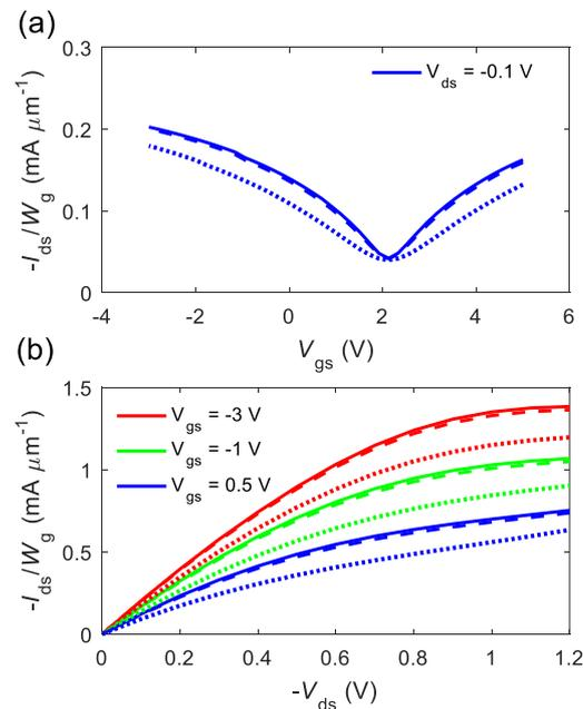
Fig. S7 Influence of interface trap density on the (a) transfer and (b) output curves. Solid lines correspond to  $N_{it} = 0 \text{ eV}^{-1} \text{ cm}^{-2}$ ; dashed lines to  $N_{it} = 10^{12} \text{ eV}^{-1} \text{ cm}^{-2}$ ; and dotted lines to  $N_{it} = 10^{13} \text{ eV}^{-1} \text{ cm}^{-2}$ .
