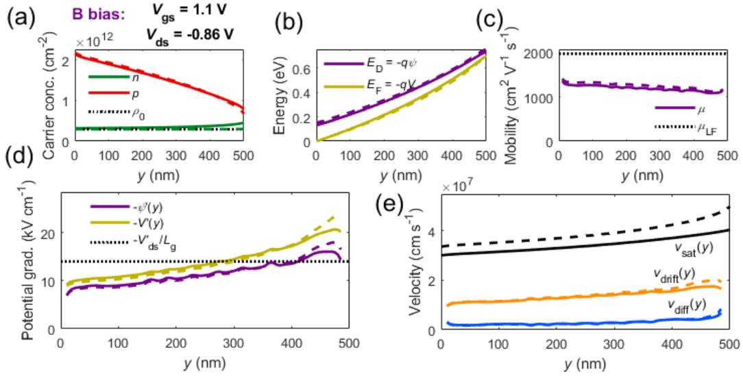
Fig. S3 Distribution along the channel of relevant parameters at bias point labelled as B in Fig. 6(a). Solid lines correspond to simulations with activated SHE ( $T = 571$  K) and dashed lines to simulations with switched-off SHE ( $T = 300$  K). (a) Electron and hole concentrations, (b) Dirac point and Fermi level, (c) field-dependent mobility (d) electric field and Fermi-level gradient, (e) saturation velocity and carrier velocity broken down into drift and diffusion velocities.
