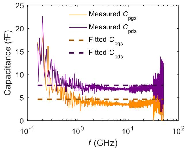
Fig. S5 Parasitic capacitances measured from the open structure of the GFET and their values obtained from  $Y$ -parameters fitting.
