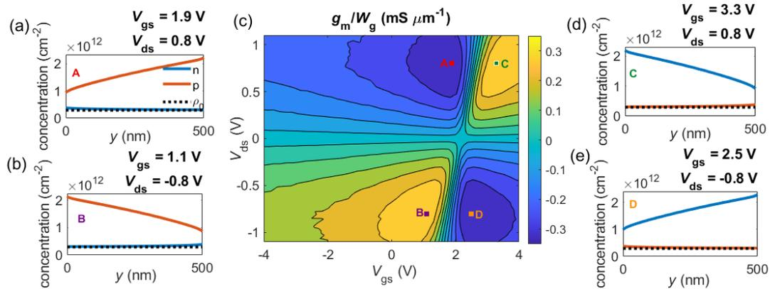
Fig. S6 Map of the bias-dependent transconductance. The map in (c) presents four maxima: (a) and (b) cases of a unipolar hole-dominated channel with the pinch-off point near the source and drain edge, respectively; and (d) and (e) cases of an electron-dominated channel near the drain and source edge, respectively. The labels A, B, C and D correspond to the bias location of the  $|g_m|$  maxima.
