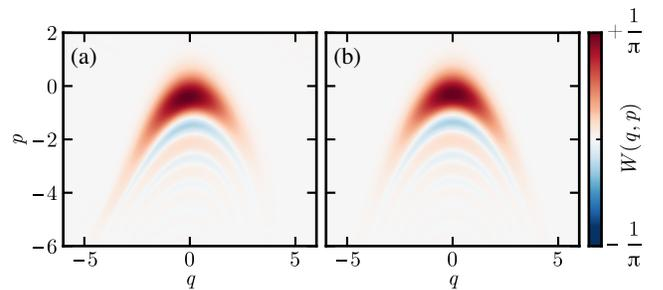
FIG. 2. Wigner distribution for the cubic phase state  $|\gamma, r\rangle$ . (a) Obtained from a master equation simulation with the Hamiltonian (5) and single-photon loss rate  $\kappa/2\pi = 50$  kHz by sequentially applying the squeezing and cubic phase gate to an initial vacuum state  $|0\rangle$  (see [46] for details). (b) Ideal cubic phase state with matched cubicity  $\gamma \approx 0.1$  and squeezing  $r \approx 0.70$  ( $\approx 6$  dB).
