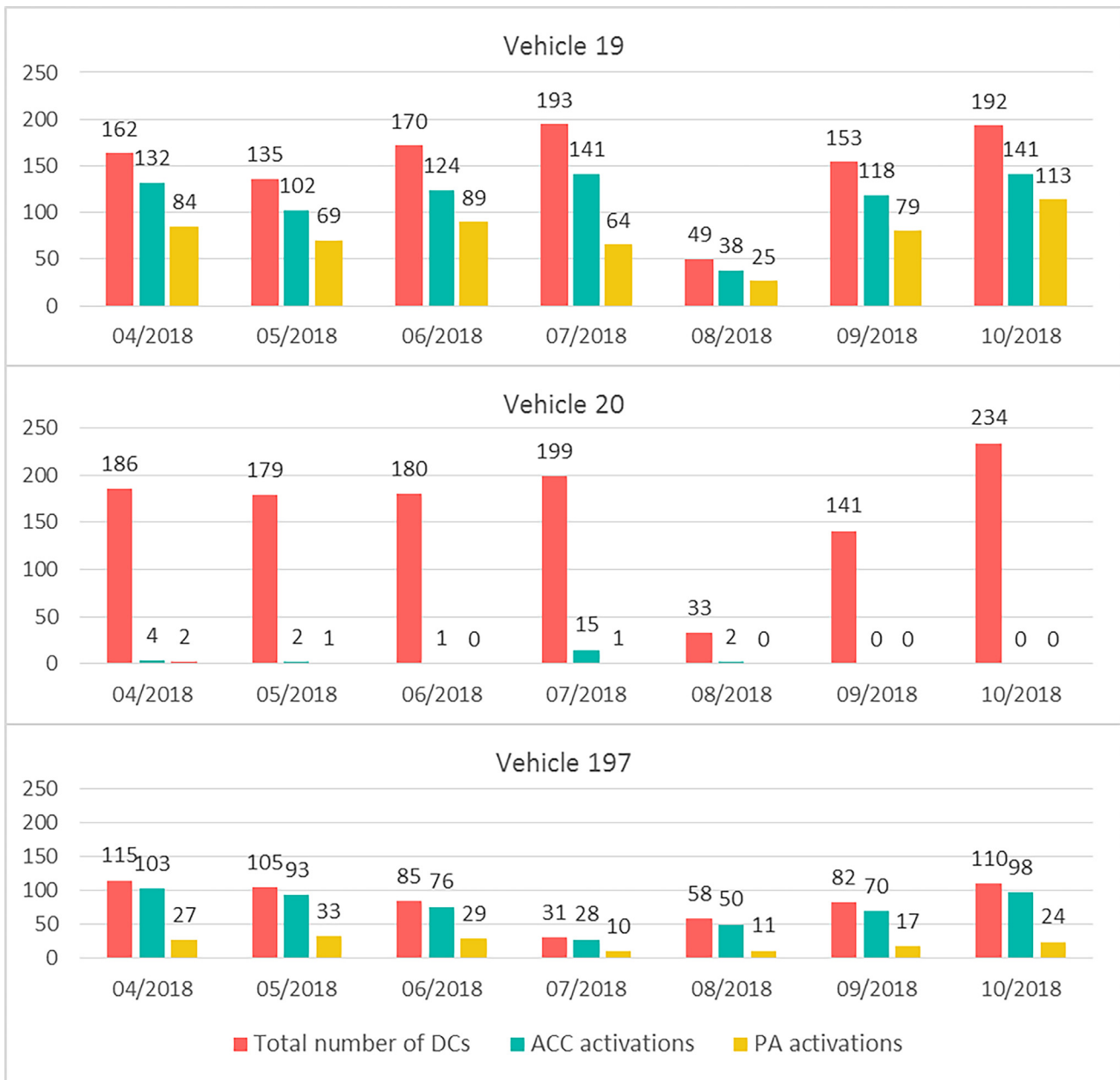
Fig. 3. Different use levels regarding ACC and PA for drivers of vehicles 19, 20 and 197.
