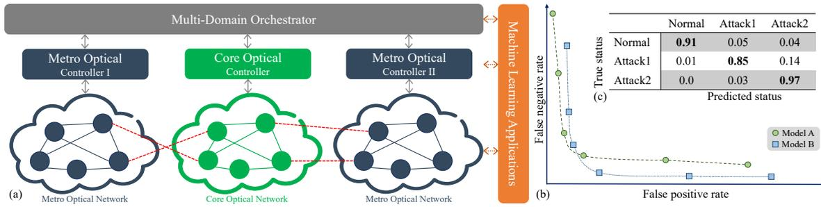
Fig. 2. (a) ML-assisted security management in multi-domain optical networks. (b) Performance trade-off among different ML models. (c) Confusion matrix for SL models.
