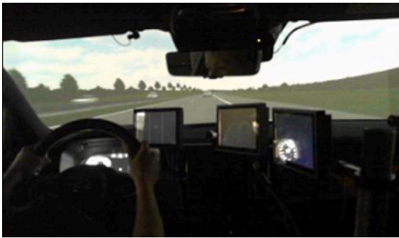
Fig. 2. Camera view of the secondary task, touch screen, monitors, steering wheel and forward roadway.
