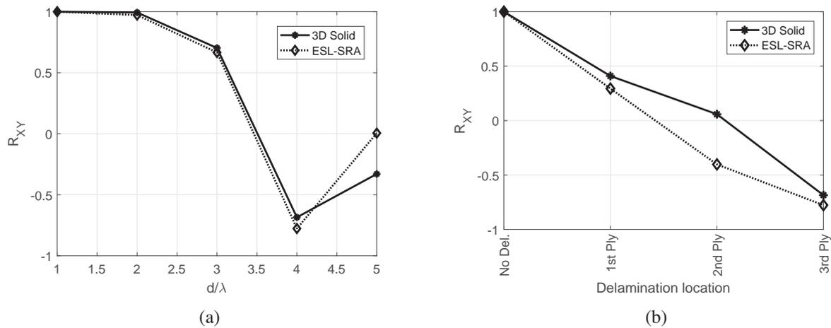
Figure 1: Effect of (a) delamination size and (b) location through the thickness on the Pearson correlation coefficient using the pitch-catch technique.
