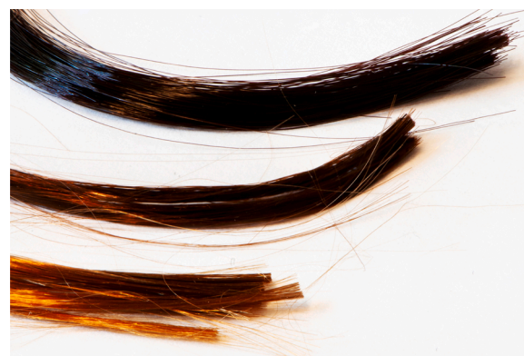
Fig. 2. Photography of three cellulose–lignin fibers. Top: 67, Mid: 33, Bot: 10 wt% lignin.
