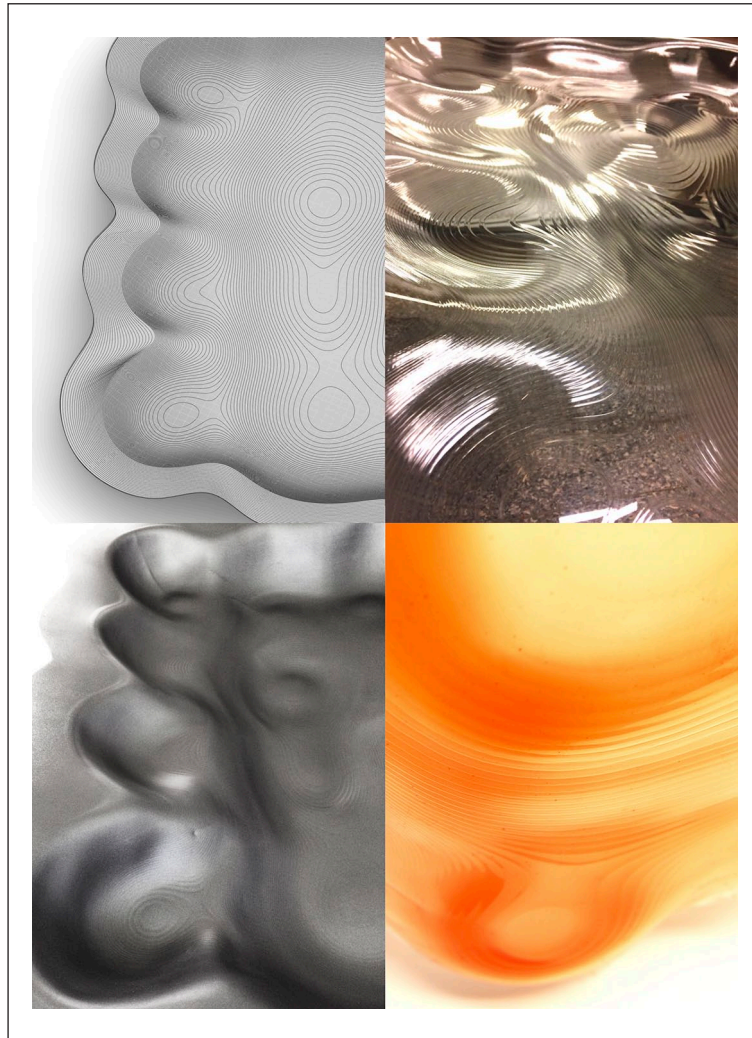
Figure 6. Differences and details arising from the transition of a digital model into a mold and into a cast in Experiment 4. Top left: Regular geometry of the toolpath for robotic incremental forming. Top right and bottom left: Geometrical imprecisions of the robotically formed mold – a deformed silhouette with local surface concavities and convexities. Bottom right: Aesthetic consequences of mold imprecision in the silicone cast – toolpath lines and varied silicone accumulations occur within the material mass, causing smooth transitions in material thickness, translucency, and color intensity.
