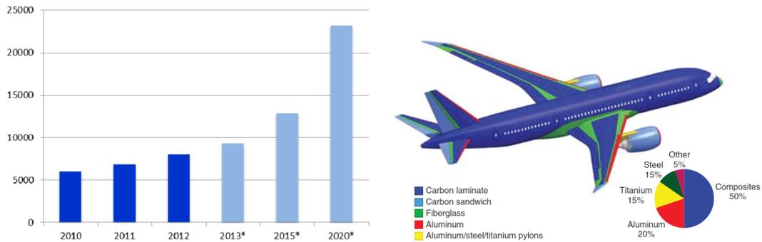
**Figure 1.2:** Carbon fibre consumption in tonnes in the market segment Aerospace Defense(\* estimated) [3] and Boeing 787 Dreamliner structural material distribution [2].
