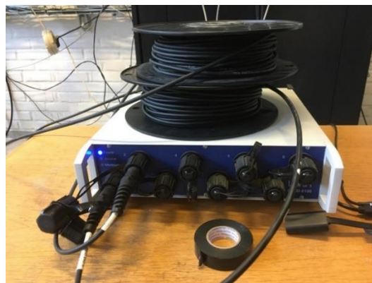
Figure 1. LUNA's ODiSI 6000 Optical Backscatter Reflectometer.
