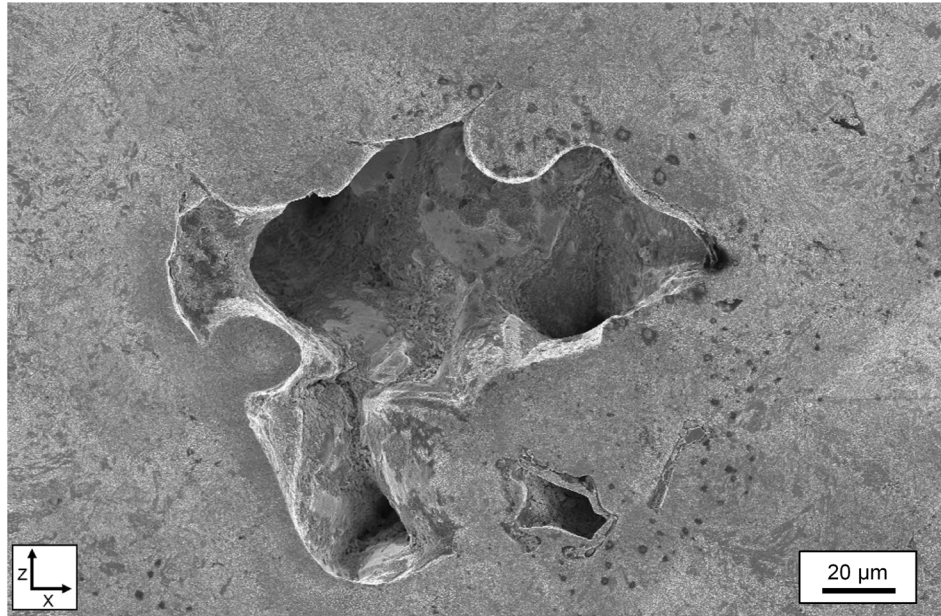
Figure 14: Lack of fusion porosity in Fe-0.2C specimen produced at 60 \text{ J/mm}^3 using a 110 W laser power.
