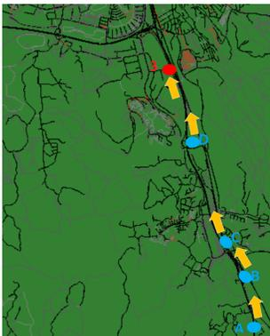
Fig. 4: Portion of Gothenburg in SUMO. The red loop detects traffic injected by blue loops.
