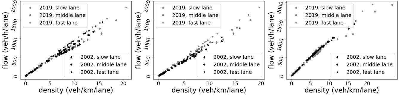
Fig. 6: Comparison of the fundamental diagrams in 2002 and 2019 passing through loops 1 (left), 2 (center) and 3 (right).
