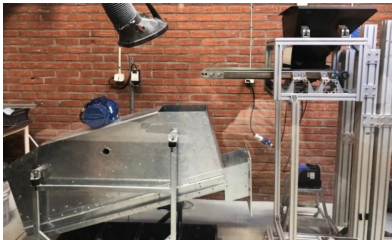
Figure 16. A photo of the laboratory-scale screen model used in experiments.
