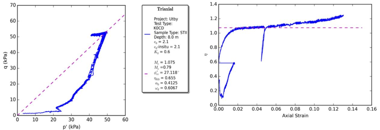
Figure 20. Drained triaxial test on Utby clay.
