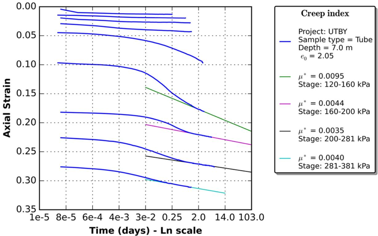
Figure 22. Modified creep index  $\mu^*$  for Utby clay.
