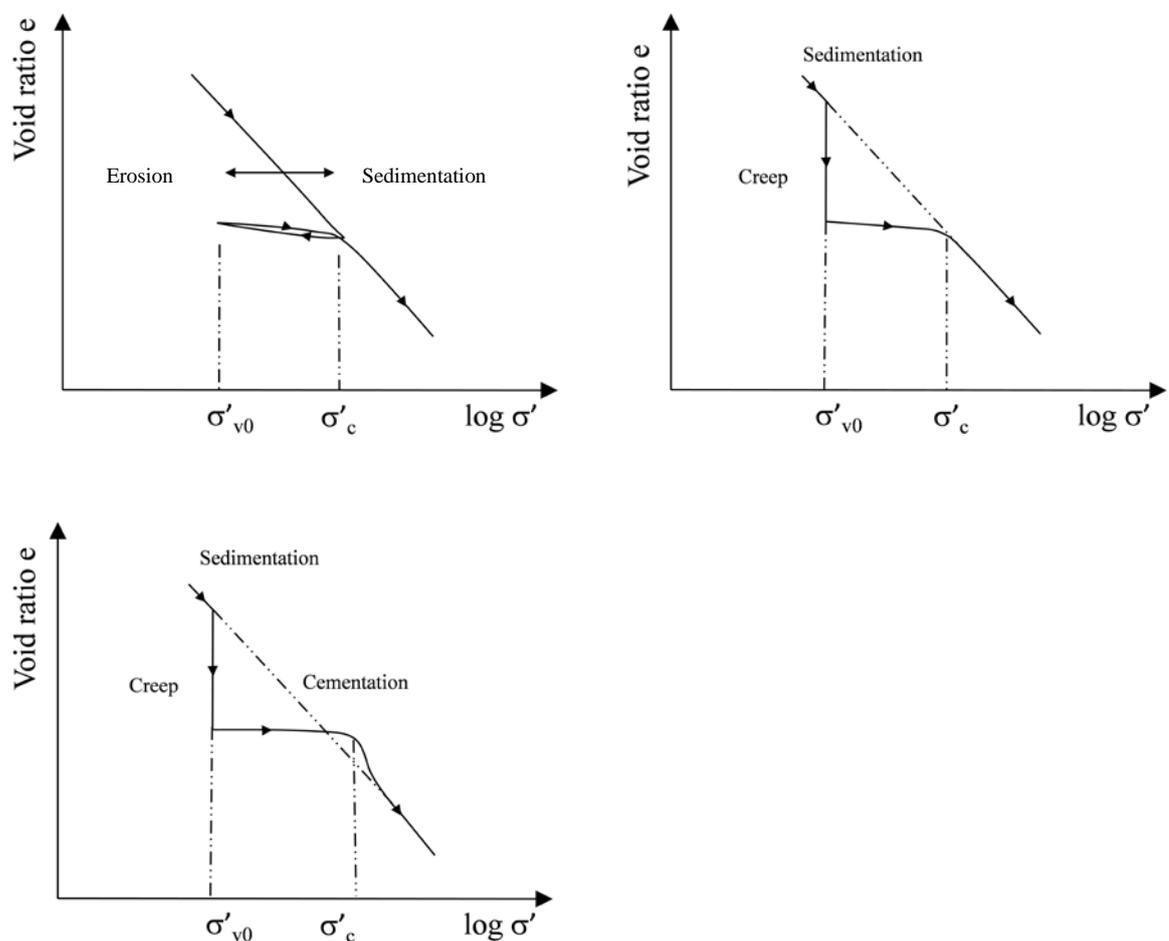
Figure 15. Effect of a) erosion, c) creep and c) creep and cementation of the apparent preconsolidation pressure.
