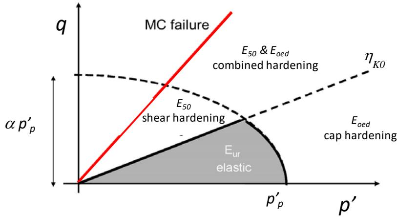
Figure 8. Yield surfaces of the Hardening Soil Model.
