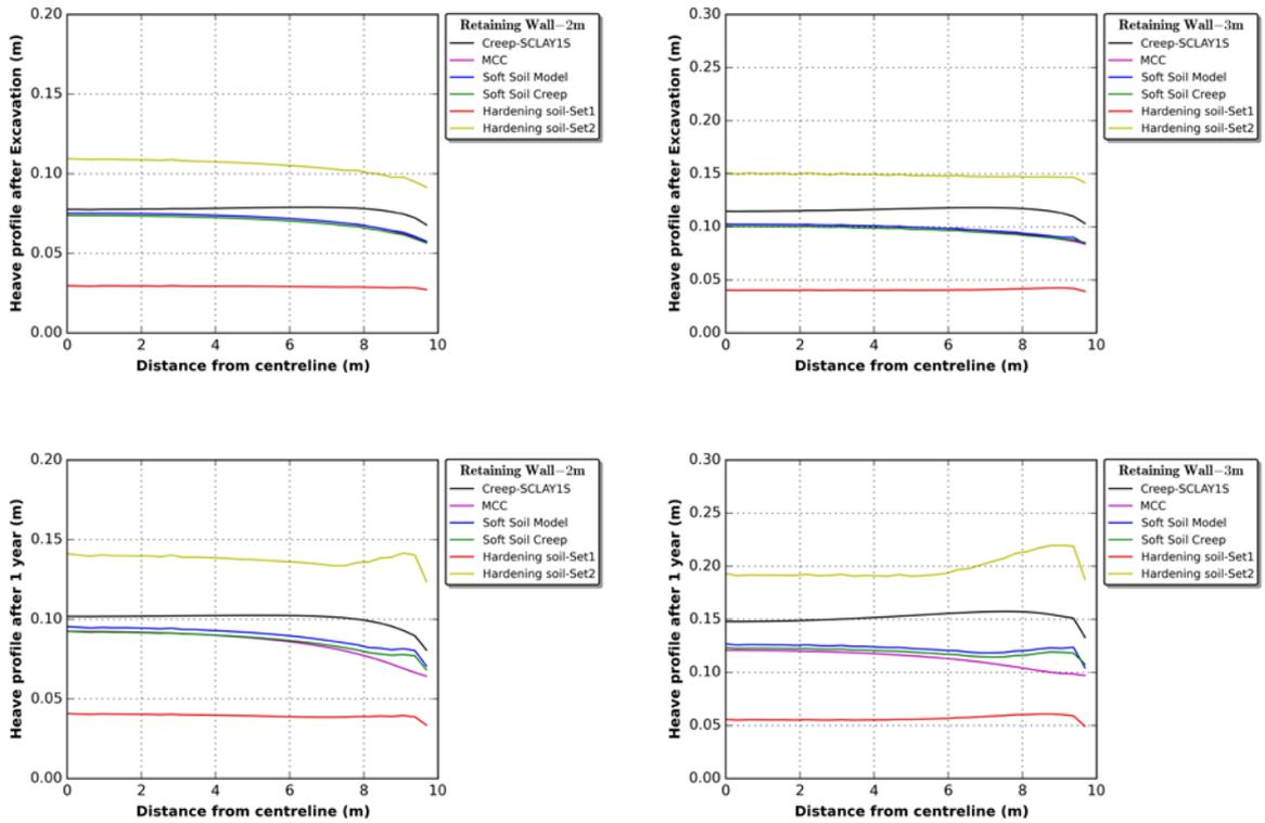
Figure 45. Predicted heave at the bottom of the excavation 2 m deep excavation (left) and for 3 m deep excavation (right).
