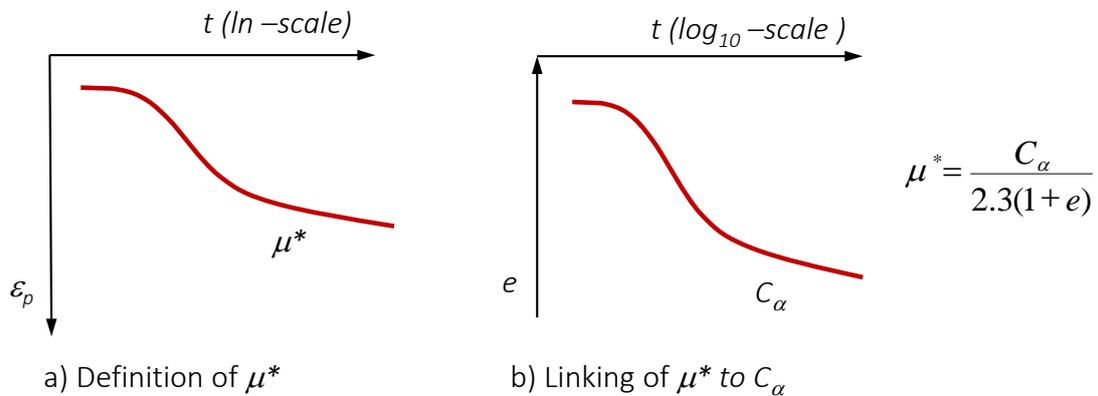
Figure 7. Definition of the modified creep index.
