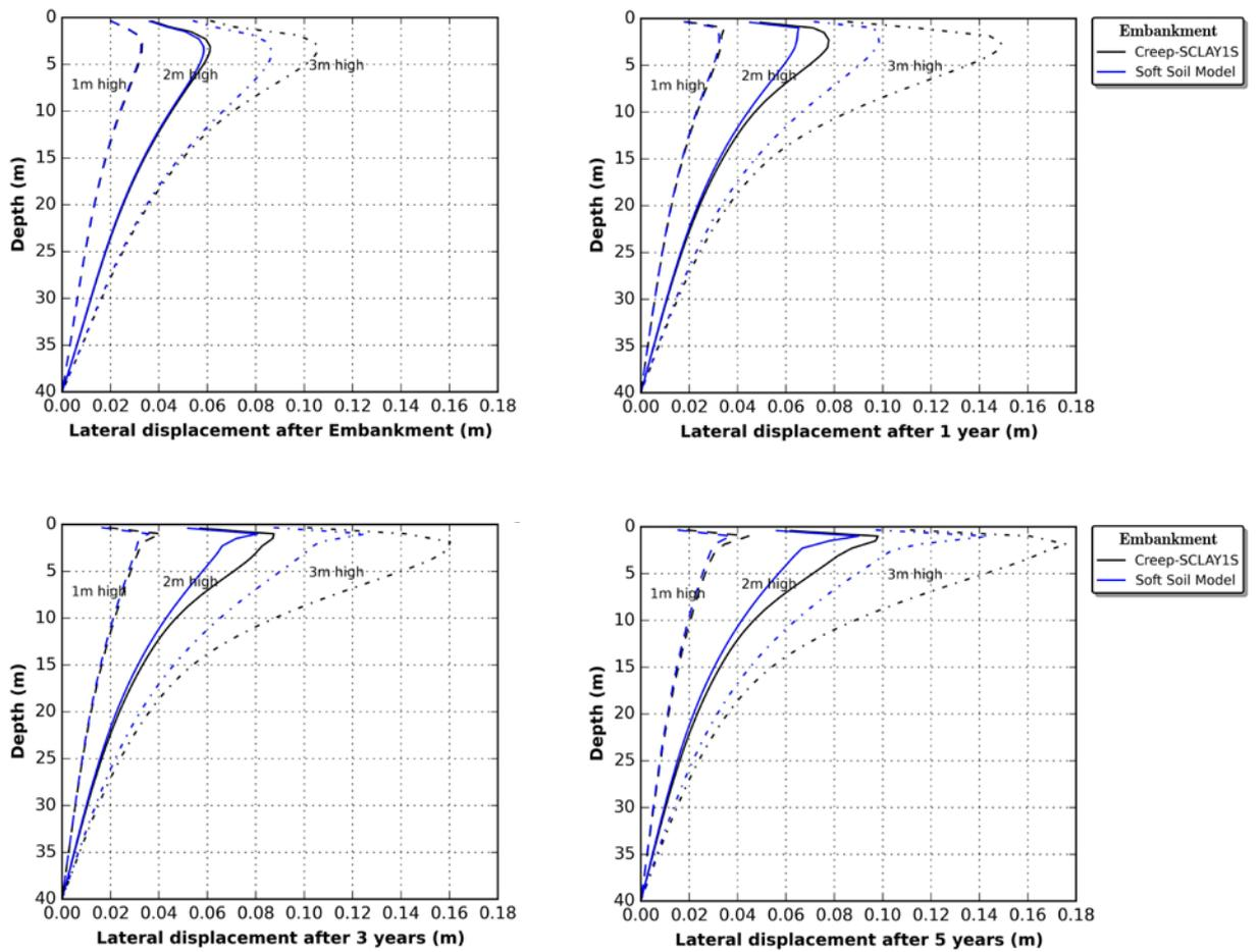
Figure 36. Predicted lateral displacement under the toe of the embankment on Utby clay: a) after construction; b) after 1 year; c) after 3 years; and d) after 5 years.
