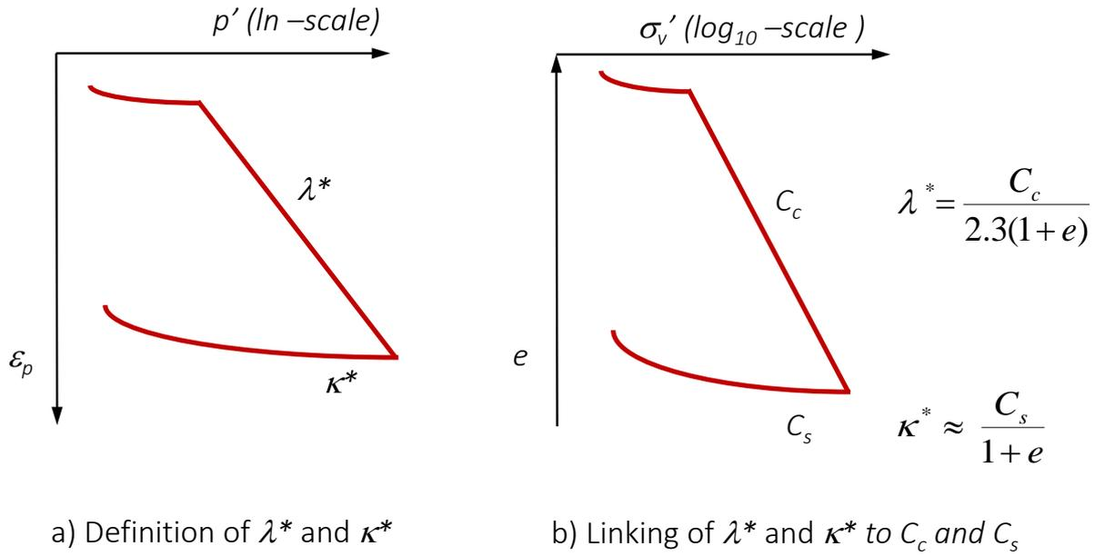
Figure 5. Definition of modified compression and swelling index.
