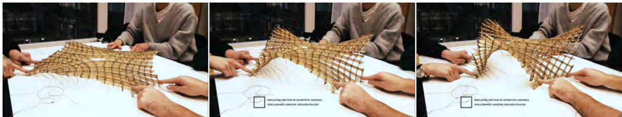
Figure 5: Physical models were made to understand the structural behaviour during erection and trying to understand the best strategy for erecting the structure. [8]
