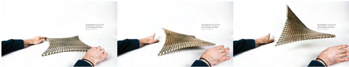
Figure 4: Small physical model of Enneper surface. It was built using planar straight 1mm plywood laths, slotted together. It can be made flat but the inbuilt energy in combination with structure being a mechanism makes it transform into an average shape between the purely geometrical and flat state[9].
