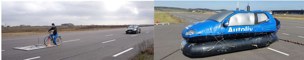
Figure 4: Dummy cyclist mounted on HSP (left) and balloon car representing the oncoming vehicle (right)
