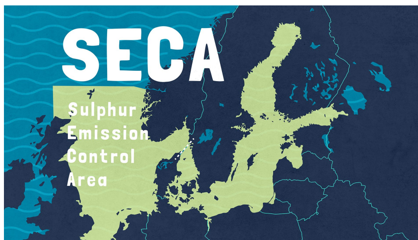
Figure 1. The European SECA which requires fuel with FSC less than 0.1% (non scrubber ships). From 2021 this area is also a NO x emission control area, requiring Tier 3 (approx. 90 % NO x abatement) for all ships from this year and onward.
