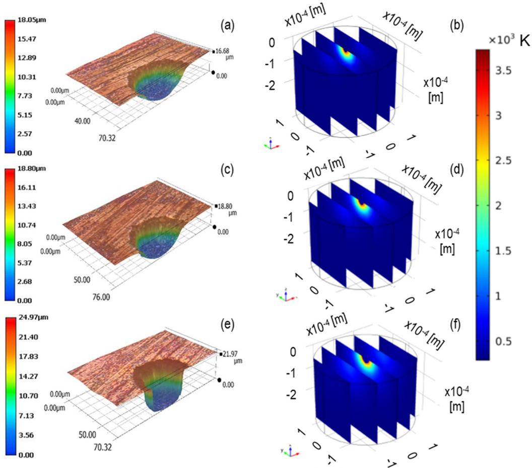
Fig. 12. Comparison between the simulation of ultra-short pulsed laser ablation of  $\text{Si}_3\text{N}_4$  and experimental results a: experimental after the 10<sup>th</sup> pulse; b: simulation after the 10<sup>th</sup> pulse; c: experimental after the 20<sup>th</sup> pulse; d: simulation after the 20<sup>th</sup> pulse; e: experimental after the 40<sup>th</sup> pulse; and f: simulation after the 40<sup>th</sup> pulse.
