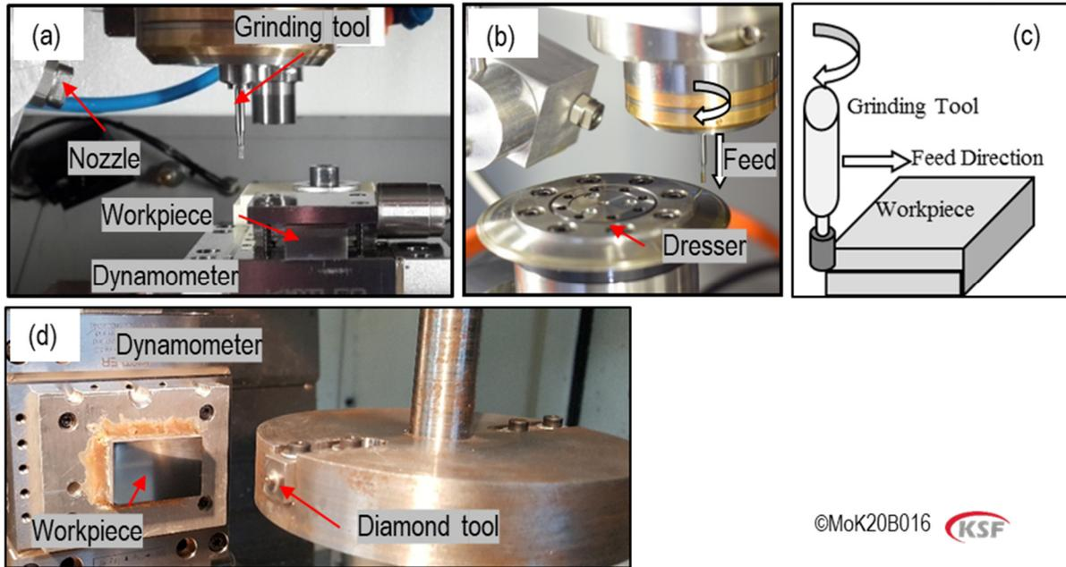
Fig. 10. a: experimental setup for the micro-grinding process; b: dressing unit and kinematic; c: schematic of peripheral surface micro-grinding; and d: experimental setup for single grain tests.
