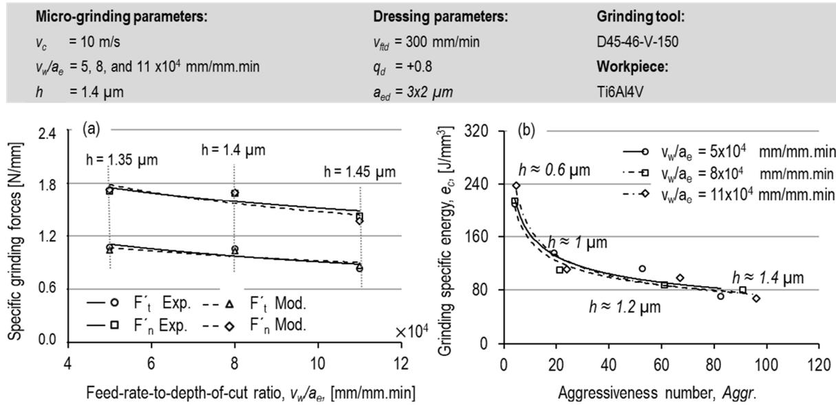
Fig. 30. The effect of  $v_w/a_e$  on a: specific grinding forces with average chip thickness of 1.4  $\mu\text{m}$  ( $a_{e-real}$  ranging from 8.1-13  $\mu\text{m}$  and  $v_w$  varying between 633-940 mm/min); and b: the grinding specific energy at different chip thicknesses ( $v_c = 10$  m/s).
