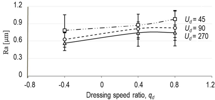
Fig. 24. Surface roughness, Ra, versus dressing speed ratio.
