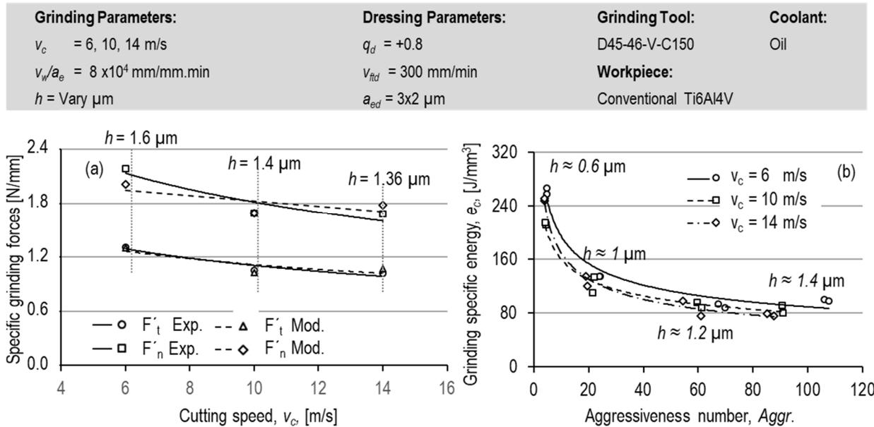
Fig. 27. The effect of cutting speed on a: specific grinding forces with average chip thickness of  $1.5 \mu\text{m}$  ( $a_e$  ranging from  $7.6\text{-}11.7 \mu\text{m}$  and  $v_w$  varying between  $347\text{-}800 \text{ mm/min}$ ); and b: the grinding specific energy at different chip thicknesses ( $v_w/a_e = 8 \times 10^4 \text{ mm/mm.min}$ ).
