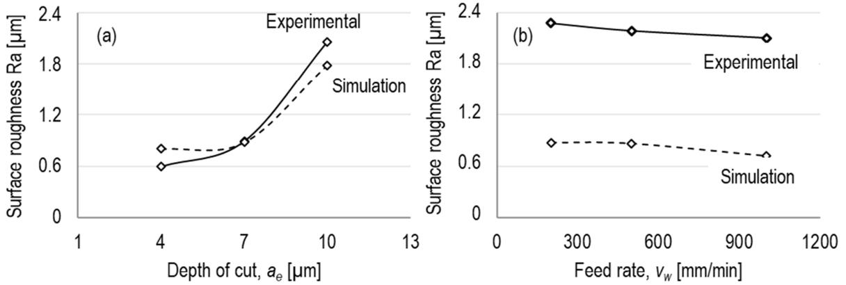
Fig. 36. The simulated and experimental values of the surface roughness versus different a: depth of cuts ( $v_c = 6 \text{ m/s}$  and  $v_w = 1000$ ); and b: feed rate ( $v_c = 14 \text{ m/s}$  and  $a_e = 7 \text{ }\mu\text{m}$ ).
