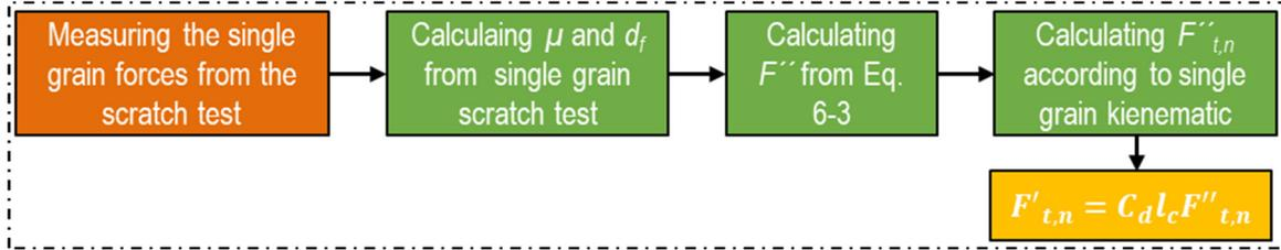
Fig. 13. The algorithm to the establishment of the single grain forces.
