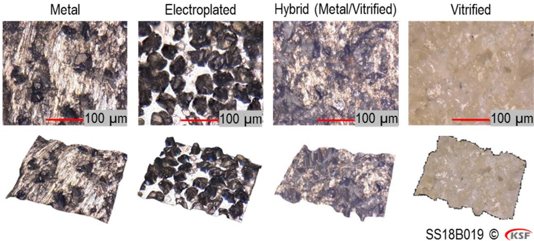
Fig. 5. Tool topography with different bonding materials [28].
