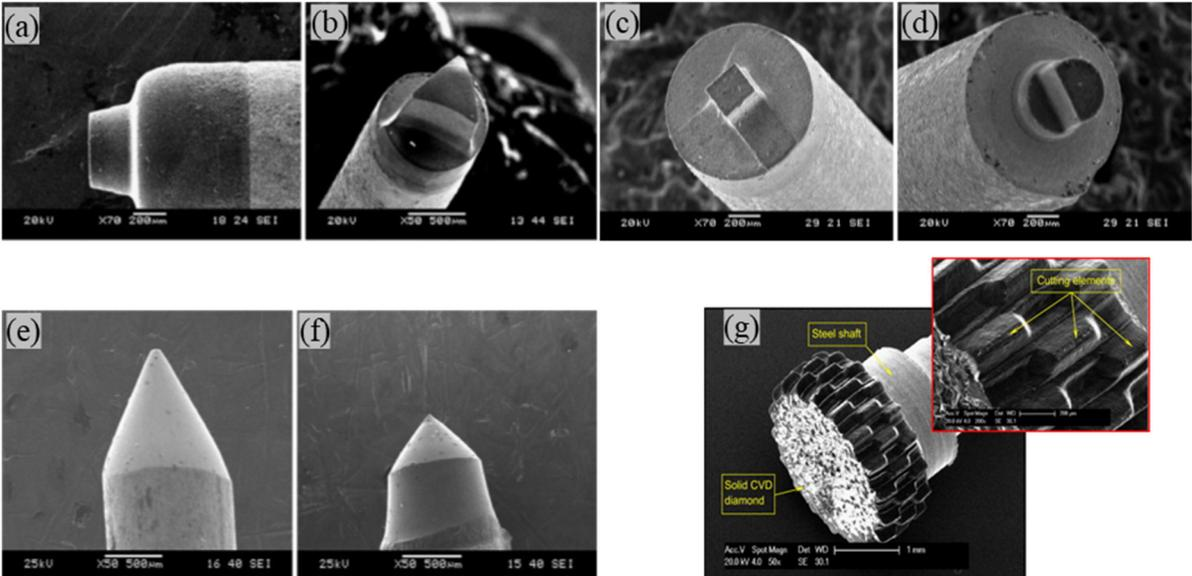
Fig. 4. Micro-grinding tools: a: circular tool; b: triangular tool, c: square tool; d: D-shaped tool; e: conical tool of 60°; f: conical tool of 90° (Reprinted by permission from [23]); and g; unused laser ablated solid diamond micro-grinding tool (Reprinted with permission from [24]).
