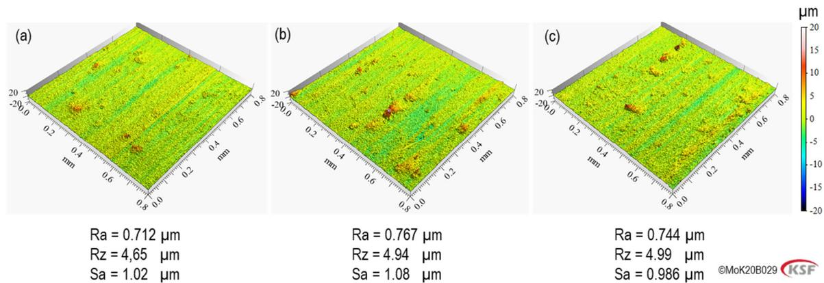
Fig. 35. Surface topography of the workpiece after micro-grinding process for a: conventional part; b: AM BD 20; and c: AM BD 30 ( $v_c = 10 \text{ m/s}$ ,  $a_e = 10 \mu\text{m}$ ,  $v_w = 800 \text{ mm/min}$ , and  $Aggr. \approx 100$ ).
