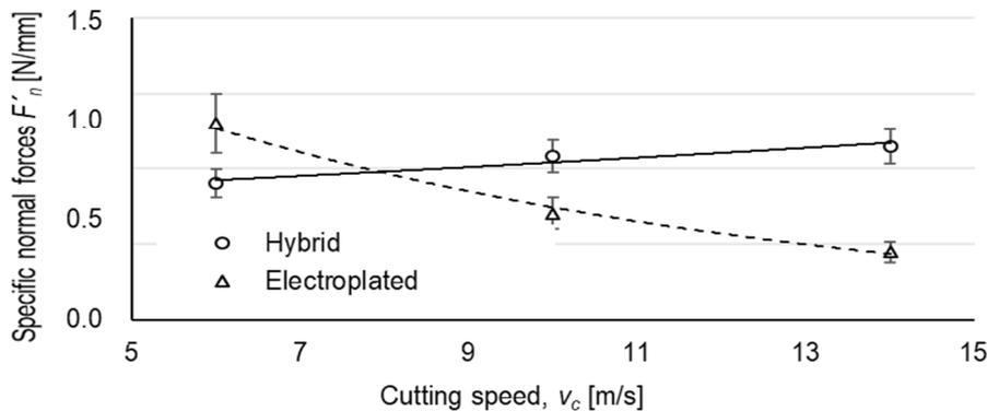
Fig. 17. The effect of cutting speed on the specific normal grinding forces.
