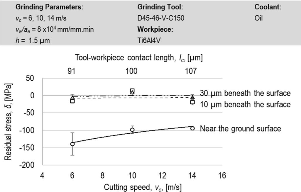
Fig. 28. The residual stress at constant chip thickness versus the cutting speed ( $v_w/a_e = 8 \times 10^4 \text{ mm/mm}\cdot\text{min}$ ).
