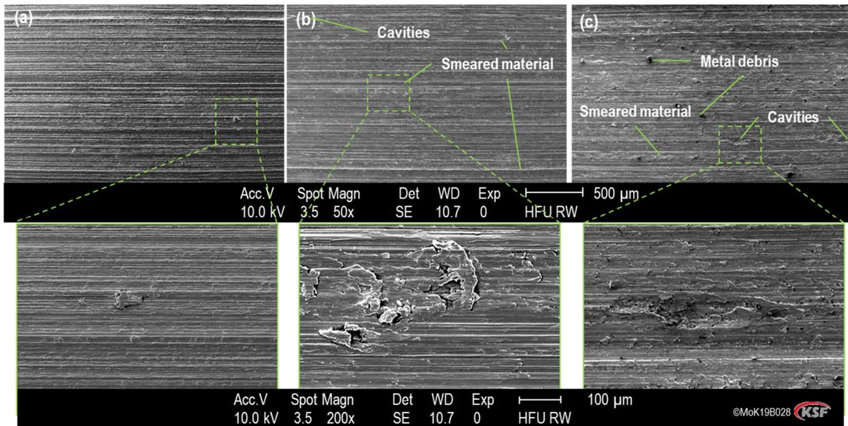
Fig. 29. Topography of the ground surface at a:  $v_c = 6$  m/s; b:  $v_c = 10$  m/s; and c:  $v_c = 14$  m/s ( $v_w/a_e = 8 \times 10^4$  mm/mm.min and  $h \approx 1.4$   $\mu$ m- *Aggr.*  $\approx 21$ ).
