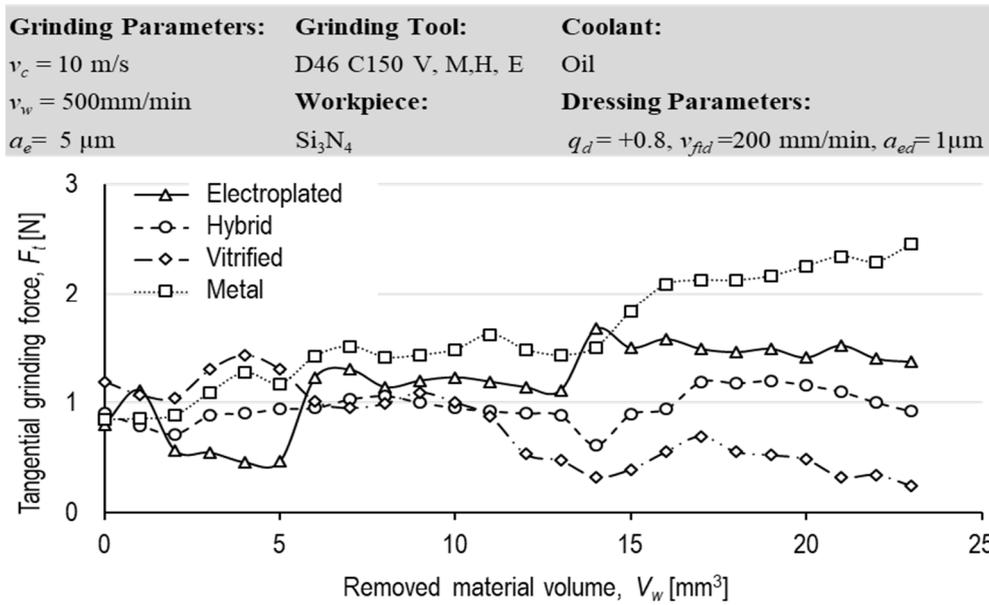
Fig. 18. Tangential grinding forces versus removed material volume.
