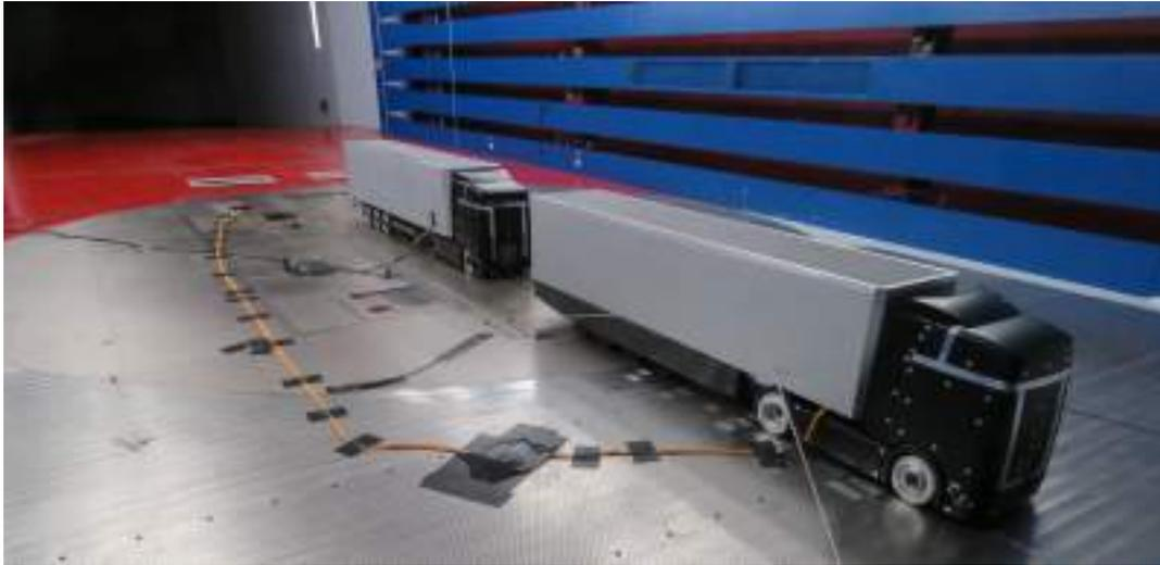
**Figure 3.13:** *Mounting solution. Here, the leading truck is the dummy model, and the trailing truck is the measurement model.*
