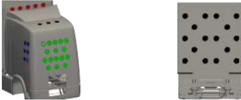
(a) Front of the truck, the colors represent the different areas of surface averaged pressure. Black: roof, Green: front, Blue: right side, Red: tractor-trailer gap.
