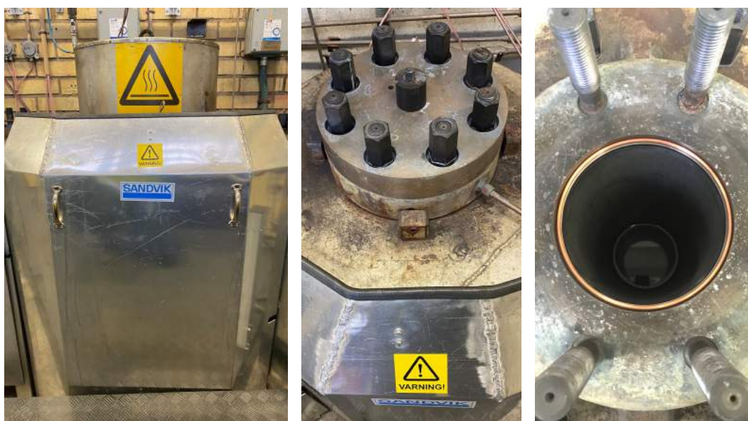
Figure 4-2: The autoclave setup: the autoclave (left), the top without cover (centre), the inside (right).
