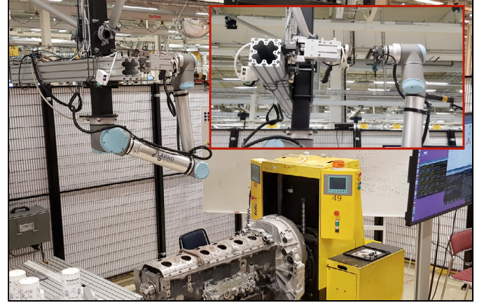
Fig. 1. Collaborative robot assembly station. Cutout at the top right highlights the tool docking mechanism. Video available at https://youtu.be/TK1Mb38xiQ8
