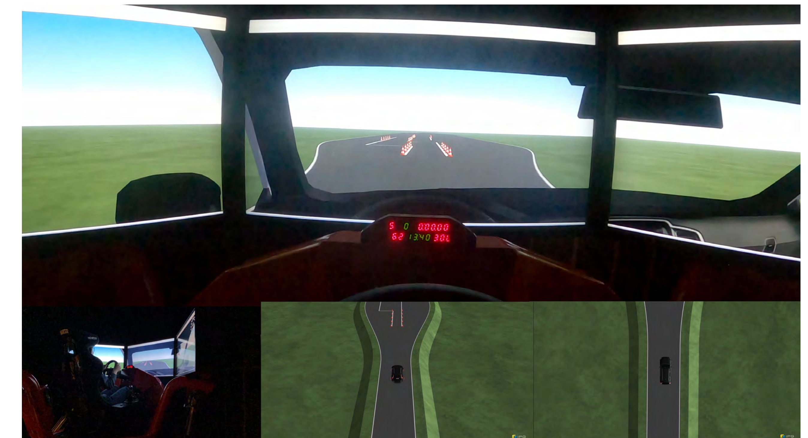
A DLC test with motion simulator
