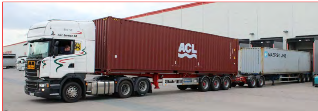
Double trailer with containers (GVW 60tonne, length 32m)
